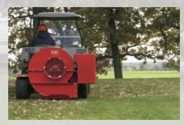
VERSATILE DESIGNS The Toro Debris Blower 400 and 600 are PTO driven models for a compact yet powerful machine. The Debris Blower 800 offers the added versatility of a self-contained, reliable power source that can be pulled behind virtually any vehicle. All models feature a 180-degree directional discharge chute that can be fully adjusted from the
