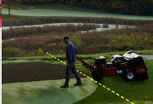
Coring head drops where aeration engaged
